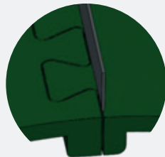
Traditional Jig-saw joint (<50% support)
